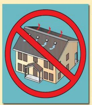
One of the most potentially troublesome attic ventilation mistakes is having two different types of exhaust vents on your house—for example, mixing a ridge vent with a powered fan, a roof louver, a gable louver or a wind turbine. Technically, this mistake is called short-circuiting the attic ventilation system. (See illustration on the left.)
